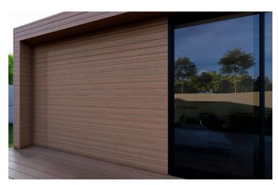
8. Continue to fit the Cladding Boards in this manner until you have completely covered the area you want. If you are running your boards length ways end to end, you will need to leave a min of 5mm gap between butt ends to allow for expansion. You may need to install more battens if you wish to do this, as each Board will need to be supported on a Batten where it meets the next Board.
