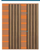
Lap the second plank into the first – the planks are designed to be interlocking and slot together along the recessed screw groove. Fix using the same method as the first panel to secure into the structural joists. Continue with subsequent planks to end of run.
