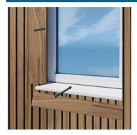
For deeper window reveals, fascia boards can be cut in length and width to finish flush with the front of the cladding panels. Secure with a high quality adhesive sealant and colour-match 35mm screws. Corners can be used in addition to 'frame' the window if required.
